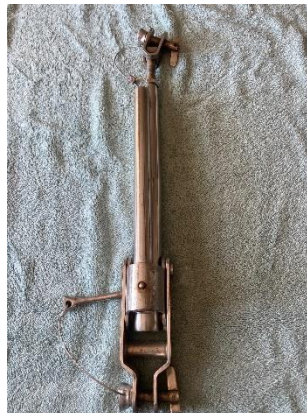
Removable stay fitting Used from Caliber 40LRC inner forestay Attached via 1/2 inch clevis pins to deck and stay - $150
