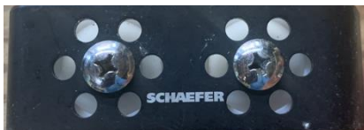
3 Series Double Deck Organizer. Sheaved for 11mm max line, $35.
